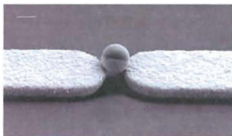
Figure 5. Micrograph of a magnetic bead bridging two \text{Ni}_{80}\text{Fe}_{20} electrodes. The scale bar is 1\ \mu\text{m} [14]. Reused with permission from [14]. Copyright 2005, American Institute of Physics.
